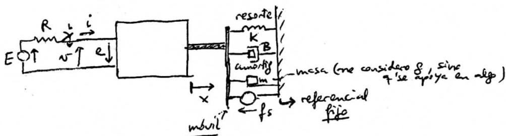
$$\left. \begin{array}{l} v = E - Ri \\ v = -e \\ e = -\frac{di}{dt} \\ f = L(x)i \end{array} \right\} \Rightarrow E = Ri + v = Ri + \frac{d}{dt} (L(x)i) = Ri(t) + \frac{d}{dt} (L(x)i(t)) + L(x)\frac{di(t)}{dt} =$$
