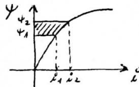
$$\Delta W_{e1 \rightarrow 2} = \int_{\psi_1}^{\psi_2} i d\psi \quad (\text{consumida, } \psi \text{ entra al convertidor})$$
