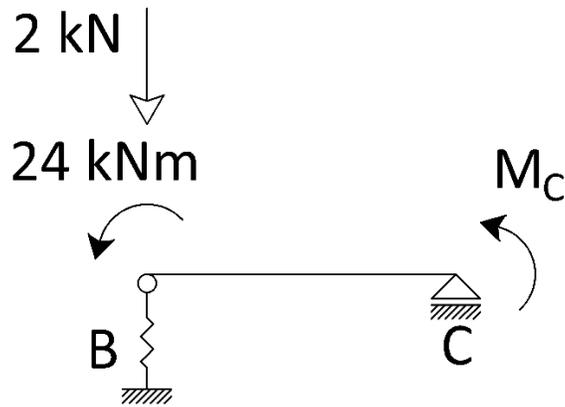
$$\theta_{F,izq} = \frac{-24 \text{ kNm } 2 \text{ m}}{6EI} + \frac{R_G}{k} \frac{1}{2 \text{ m}} + \frac{M_C 2 \text{ m}}{3EI}$$
