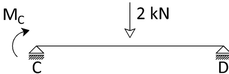
$$\theta_{der} = \frac{M_C 4 \text{ m}}{3EI} + \frac{2 \text{ kN } (4 \text{ m})^2}{16EI}$$
