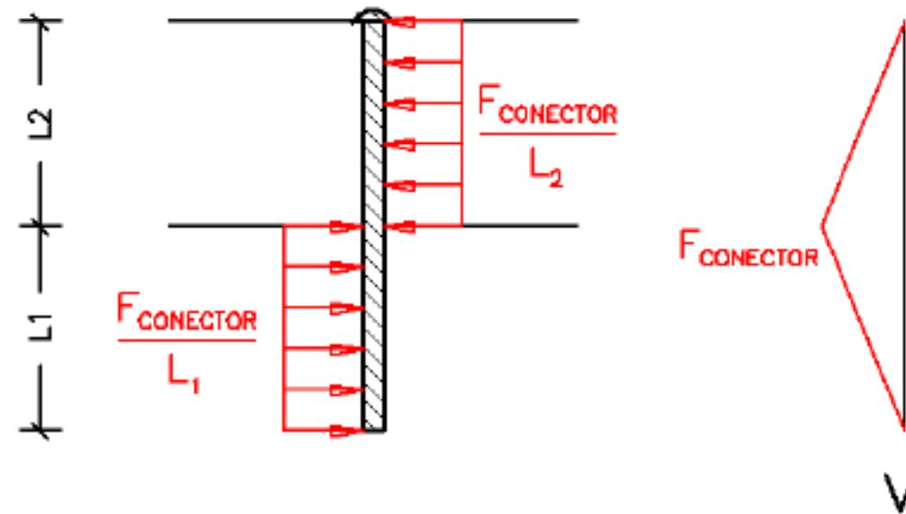
$$V_{conector}^{m\acute{a}x} \text{ (corte simple)} = F_{conector}$$
