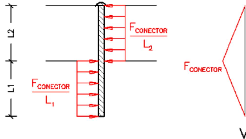
$$V_{conector}^{m\acute{a}x} \text{ (corte simple)} = F_{conector}$$
