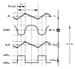
Figure 15.3. Forward converter, three output ripple components, showing: left -voltage components; centre - waveforms; and right - capacitor model.
