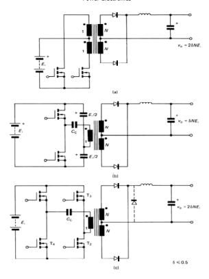
Figure 15.15. Multiple-switch, isolated output, pulse-width modulated converters:
