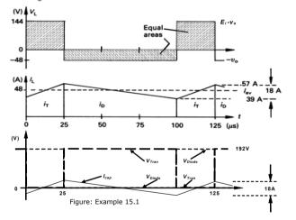
iv. Current  $i_D$  through diode D is shown on the inductor current waveform. The average diode current is
