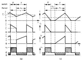
Figure 15.5. Non-isolated, step-up, flyback converter (boost converter) where  $v_0 \ge E_i$ :
