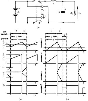
Figure 15.7. Basic reversible converter with  $\delta > \frac{1}{2}$ :
