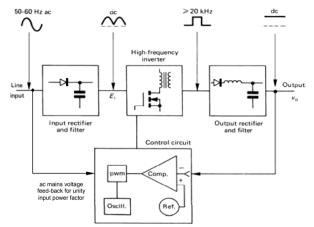
Figure 15.1. Functional block diagram of a switched-mode power supply.
