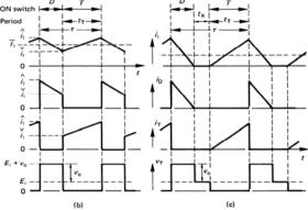
Figure 15.6. Non-isolated, step up/down flyback converter (buck-boost converter) where v₀ ≤ 0: (a) circuit diagram; (b) waveforms for continuous inductor current; and (c) discontinuous inductor current waveforms.
