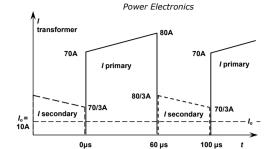
Figure 15.12. Currents for the transformer windings in example 15.7.
