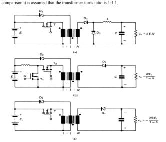
Figure 15.10. Isolated output versions of the three basic converter configurations: (a) the forward converter; (b) step-up flyback converter; and (c) step up/down flyback converter.
