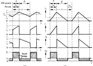
Figure 15.2. Non-isolated forward converter (buck converter) where  $v_0 \le E_1$ : (a) circuit diagram; (b) waveforms for continuous output current; and (c) waveforms for discontinuous output current.
