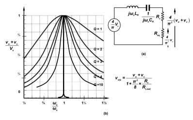
Figure 15.18. Series resonant converter (a) equivalent circuit and (b) normalised output voltage curves.
