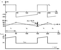
Figure: Example 15.3 - waveforms
