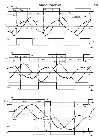
Figure 15.22. Three modes of parallel load resonant converter operation: (a)  $f_s > f_{o'}$  (b)  $\frac{1}{2}f_o < f_s < f_{o'}$  and (c)  $f_s < \frac{1}{2}f_{o'}$ .
