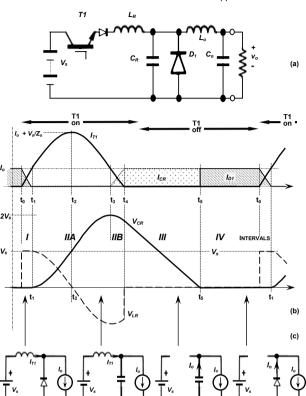
Figure 15.24. Zero current switching, ZCS, resonant switch dc to dc converter: (a) circuit; (b) waveforms; and (c) equivalents circuits.
