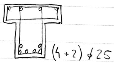
$$c) q_d = 97,20 \text{ kN/m} \Rightarrow M_d = \frac{97,20 \times 6,4^2}{8} = 497,66 \text{ kNm}$$
