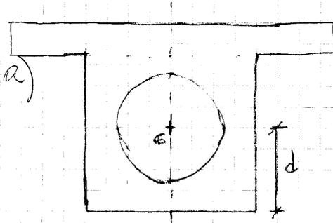
$$i) u_G = 150 \times 15 \times 82,5 + 77,5 \times 80 \times 75 - d \frac{\pi 75^2}{4} = d (15 \times 150 + 80 \times 75 - \frac{\pi 75^2}{4})$$
