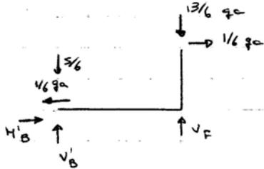
$$\left\{ \begin{aligned} H'_B &= 0 \\ V'_B + V_F &= 3qa \\ V_F 2a - \frac{3}{2} qa 2a - \frac{1}{2} qa a &= 0 \Rightarrow V_F = \frac{1}{4} qa \\ V'_B = (3 - \frac{1}{4}) qa &= \frac{11}{4} qa \end{aligned} \right.$$
