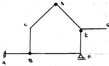
$$\left\{ \begin{aligned} H_B &= H_E \\ V_B + V_E &= 3qa \\ V_B 2a + H_B a &= \frac{3}{2} qa^2 \\ V_B a + H_B 2a &= \frac{9}{2} qa^2 \end{aligned} \right.$$
