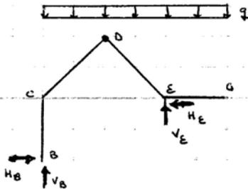
$$\begin{aligned} 2V_B + H_B &= 3/2 qa \\ -2V_B + 2H_B &= -qa \\ 3H_B &= 1/2 qa \\ H_B = H_E &= 1/6 qa \\ V_B = \frac{3qa}{2} + 2H_B &\Rightarrow V_B = \frac{5}{2} qa \\ V_E = 3qa - V_B &\Rightarrow V_E = \frac{1}{2} qa \end{aligned}$$
