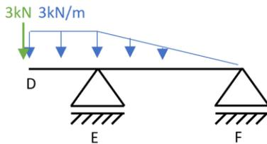
$$\Sigma M_F = 0 \Rightarrow V_E \cdot 3m = 3kN \cdot 4m + \frac{3kN}{m} \cdot 1m \cdot 3,5m + \frac{3kN}{m} \cdot \frac{3m}{2} \cdot 2m \Rightarrow V_E = 10,5kN$$
