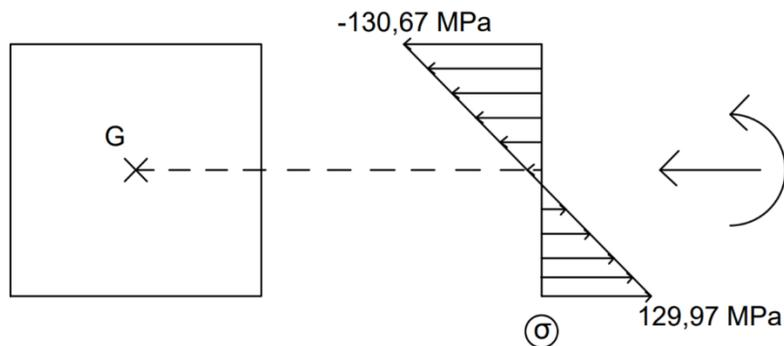
$$\sigma_{comp} = \frac{M_{m\acute{a}x}}{W} + \frac{N}{A} = \frac{381,75 \text{ kNm}}{2,93 \times 10^{-3} \text{ m}^3} + \frac{23,5 \text{ kN}}{0,0676 \text{ m}^2} \cong 130,67 \text{ MPa}$$
