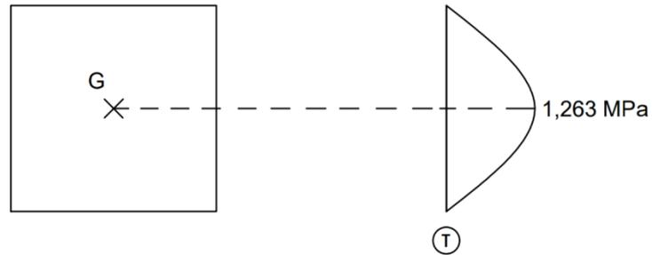
$$\tau_{m\acute{a}x} = \frac{V_{m\acute{a}x} \cdot \mu_G}{I_x \cdot b} = \frac{56,92 \text{ kN} \cdot (a \cdot a/2 \cdot a/4)}{(a^4/12) \cdot a} = \frac{56,92 \text{ kN} \cdot 2,197 \times 10^{-3} \text{ m}^3}{3,808 \times 10^{-4} \text{ m}^4 \cdot 0,26 \text{ m}} \cong 1,263 \text{ MPa}$$
