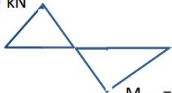
$$M_{\max} = x/2 \cdot (+10 \text{ kN} - 20 \text{ kN} \cdot (4-x)/x)$$
