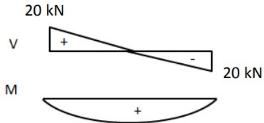
$$M_{\max} = 10 \text{ kN.m} = 20 \text{ kN} \cdot 1\text{m}/2$$
