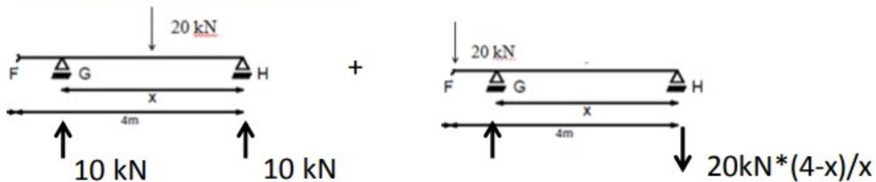
$$R_H = 10 \text{ kN} - 20 \text{ kN} \cdot (4-x)/x$$
