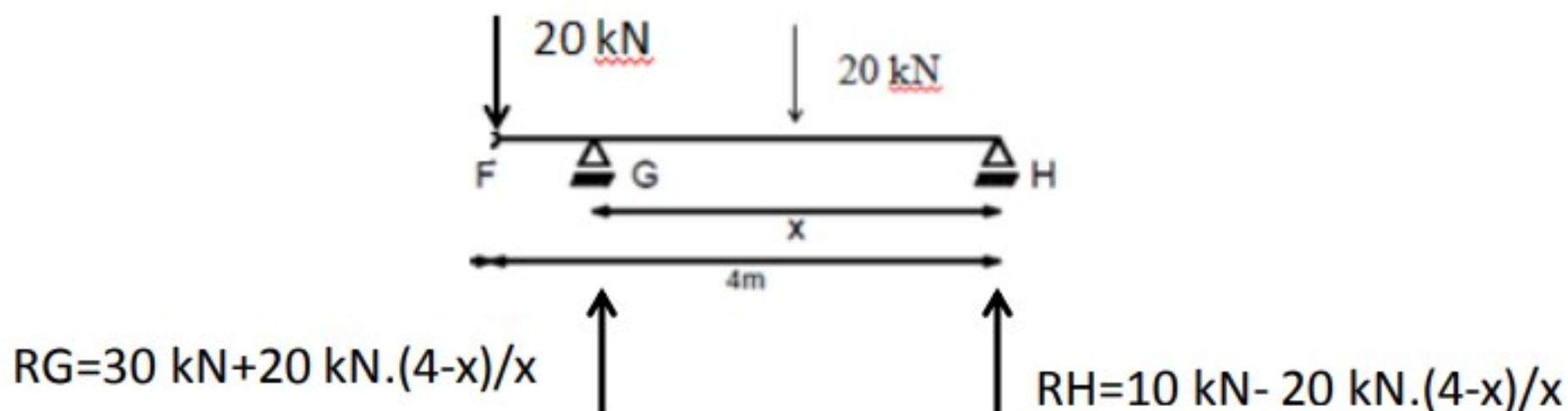
$$R_G = 30 \text{ kN} + 20 \text{ kN} \cdot (4-x)/x$$
