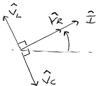
$$2) \quad Z_{eq} = R + j\omega L + \frac{1}{j\omega C} \Rightarrow \hat{I} = \frac{V_0 e^{j\omega t}}{Z_{eq}}$$
