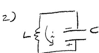
$$L \frac{di}{dt} + \frac{q}{C} = 0 \quad ; \quad i = \frac{dq}{dt} \Rightarrow L \frac{d^2q}{dt^2} + \frac{1}{C} q = 0$$
