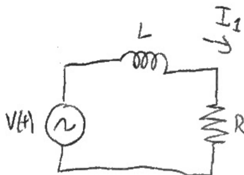
$$V(t) = V_0 \cos(\omega t) \rightarrow V(t) = \operatorname{Re} \left\{ V_0 e^{j\omega t} \right\}$$
