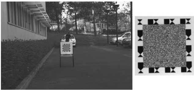
Fig. 10 Real camera example. Taken at f/5.7 . An example image, to show how local the PSF estimation is (left), and a zoom of the observed window of size 110 \times 110 pixels (right)
