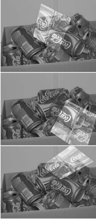
Figure 26. “Coca-Cola” experiment: registration with respect to the meaningful groups. Because there are several affine matches per group, one can compute the best planar projective mapping by a standard least squares method. The projective transformation is used to superpose the two images (on the left). On the right side, pieces of level lines that are close to each other in the registered images (see text).
