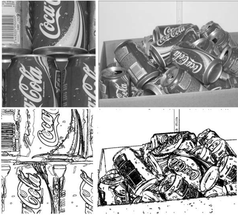
Figure 22. “Coca-Cola” experiment: original images and maximal meaningful level lines. Top: images, bottom: meaningful level lines [5].
