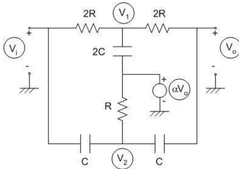
$$\left\{ \begin{array}{l} \text{Nudo } V_1 \\ \text{Nudo } V_2 \\ \text{Nudo } V_o \end{array} \right. \left\{ \begin{array}{l} \frac{V_i - V_1}{2R} = 2C\omega j(V_1 - \alpha V_o) + \frac{V_1 - V_o}{2R} \\ C\omega j(V_i - V_2) = \frac{V_2 - \alpha V_o}{R} + C\omega j(V_2 - V_o) \\ \frac{V_1 - V_o}{2R} = C\omega j(V_o - V_2) \end{array} \right.$$
