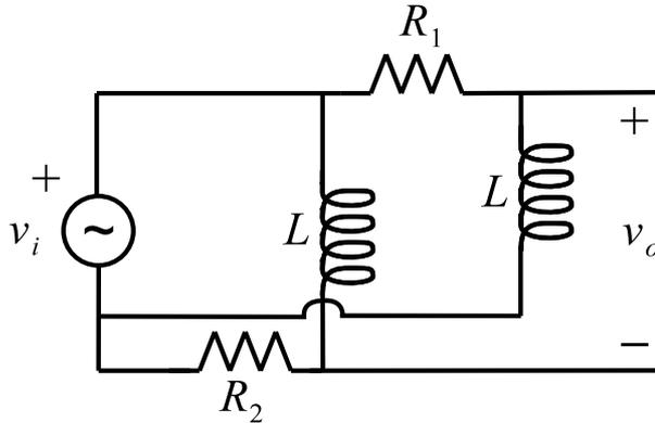
$$\begin{aligned} R_1 &= 100R \\ R_2 &= R \\ \omega_0 &= \frac{R}{L} \end{aligned}$$
