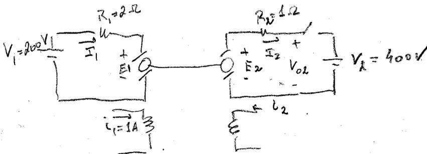
1)  $V_{02} = 405 \text{ V} = E_2$        $P_2 = E_2 I_2 = 0$       pues  $I_2 = 0$
