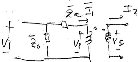
$$\left\{ \begin{array}{l} \frac{\bar{V}_p}{N_1} = \frac{\bar{V}_s}{N_2} \\ N_1 \bar{I}_1 = N_2 \bar{I}_2 \\ R = R_1 + \left( \frac{N_1}{N_2} \right)^2 R_2 \\ X = X_1 + \left( \frac{N_1}{N_2} \right)^2 X_2 \end{array} \right.$$
