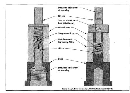
Silicon crystal rectifiers played an important role in World War II as the key components of radar receivers. These drawings are cross sections of crystal rectifier cartridges produced by Sylvania [left] and Western Electric [right] during World War II.
