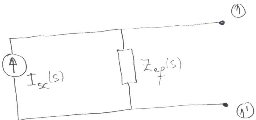
$$I_{sc}(s) = \frac{E_{oc}(s)}{Z_{ef}(s)} = \frac{\gamma}{4R} \cdot \frac{1}{(2s+1)} (sV_s(s) + 2N_{01})$$
