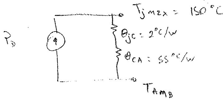
$$\Rightarrow T_{amb_{max}} = T_{jmax} - (\theta_{jc} + \theta_{ca}) P_D = 12,6^\circ\text{C}$$
