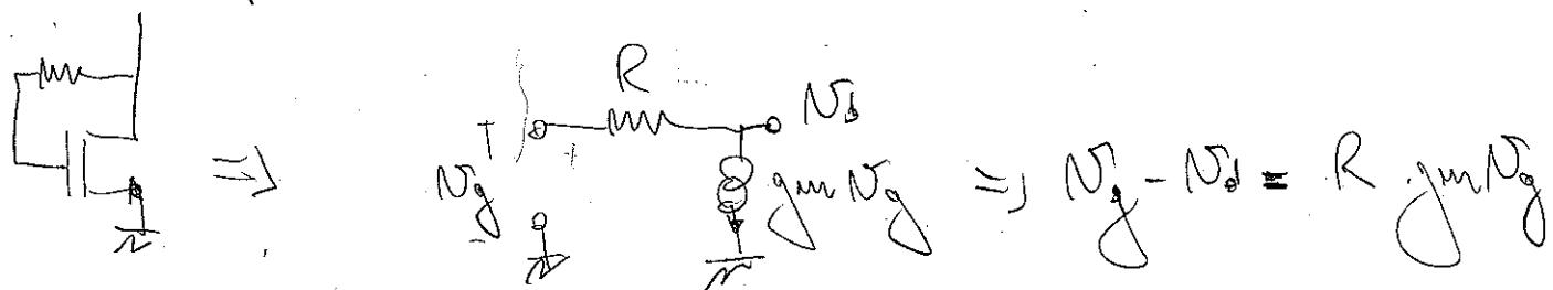
$$\Rightarrow \frac{N_d}{N_g} = (1 - R g_m) \Rightarrow V_{gp} = (1 - R g_m) V_{gp}$$
