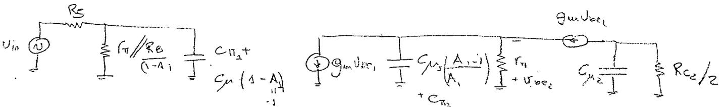
$$f_3 = \left[ (C_{\pi 1} + 2C_{\mu 1}) \left( \frac{R_B}{1-A} // R_s // r_{\pi} \right) \right]^{-1} \frac{1}{2\pi} = \left[ (1.75p + 10p) \cdot 55 \right]^{-1} \frac{1}{2\pi} = 240 \text{ MHz}$$
