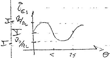
$P_S^+ = \frac{V_{cc}}{2\pi} \int_0^{2\pi} i_{c1} d\theta = \frac{V_{cc}}{2\pi} \int_0^{2\pi} (I_0 + \frac{\hat{V}_o}{R_L} \sin \theta) d\theta = V_{cc} I_0$
