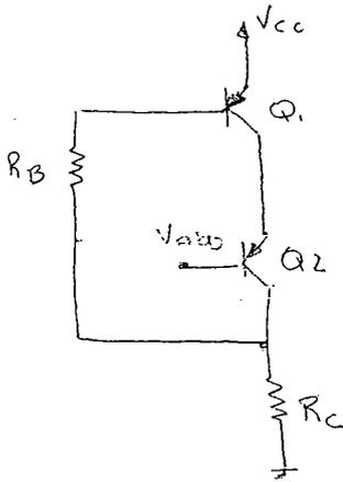
$$V_{CC} = V_{BE} + R_B I_B + R_C (I_E + I_C) \stackrel{\substack{I_B = I_C/\beta \\ I_E = I_C/\beta + I_C}}{=} V_{BE} + R_B \frac{I_C}{\beta} + R_C I_C$$
