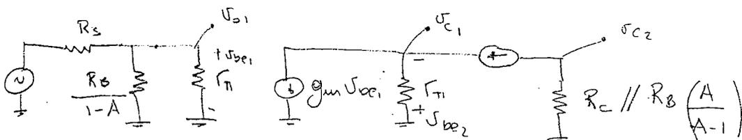
$$A = \frac{V_{C2}}{V_{B1}}$$
