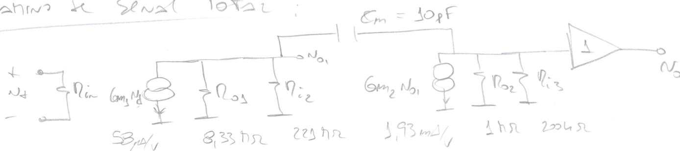
$\Rightarrow A_D = g_{m1} \cdot (R_{L1} // R_{i2}) \cdot g_{m2} (R_{L2} // R_{i3})$
