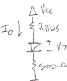
$$I_o = 1 \text{ mA} \Rightarrow \frac{V_{ce} - I_c 500 \text{ mV} - V_B}{R_{B12S}} = 1 \text{ mA} \Rightarrow R_{B12S} = \frac{V_{ce} - 1 \text{ mA} 500 \text{ mV} - V_B}{1 \text{ mA}} = 13.9 \text{ K}\Omega$$
