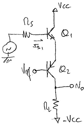
$$(e) \underline{DC}: V_{E1} = V_{S2} = V_{REF} + V_{EB} = -0,8V$$
