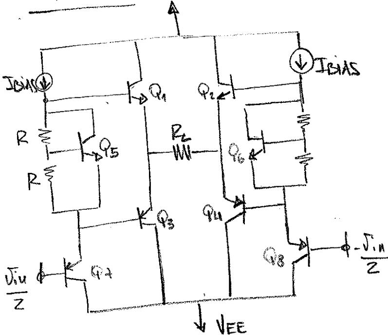
$$\textcircled{a} \quad I_{RL\max} | \quad I_{BIAS} = \frac{V_{EE}}{R} + \frac{I_{RL\max}}{\beta_1}$$
