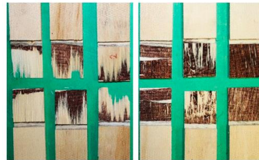
Figure 6. Amount of the wood failure in some of the shear strength samples at 45% T+P+4% BA: (left) air conditioned status; (right) after 24 h immersion in water.
