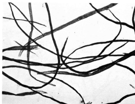
Figure 7a. Southern pine kraft, sheet pulp, not fluffed (X50).
