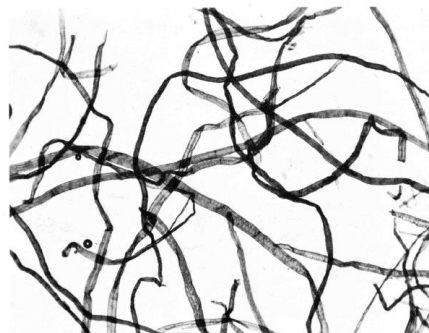
Figure 8a. Western hemlock sulfite, sheet pulp, not fluffed (X50).
