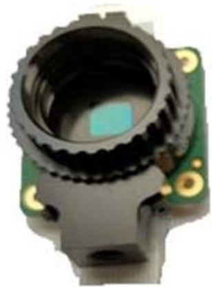
Raspberry Pi HQ Camera Sensor IMX477 → 12,3 Mpx.
