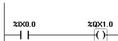
4. The Connecting Line between the Contacts and the Coils.
