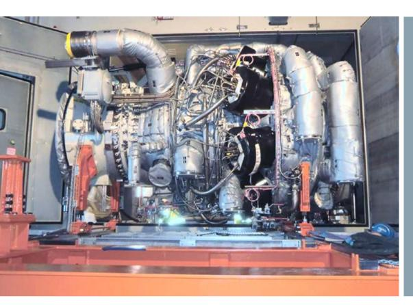
The SGT-750 gas generator can be swapped in less than 24 hours. The gas generator is rolled out with standard maintenance tools.
