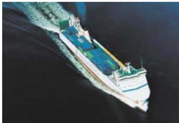
The Ro-Ro vessel Seagard is powered by one Wärtsilä 16V46, output 15 600 kW at 500 rpm and equipped with Direct Water Injection.
