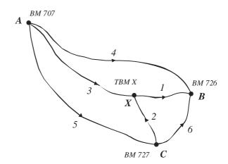
There are n = 6 levelled height differences (observations) and only  $n_0 = 3$  observations are required to determine the heights of all points, hence there are  $r = n - n_0$  redundant measurements, which is equal to the number of independent observation equations.
