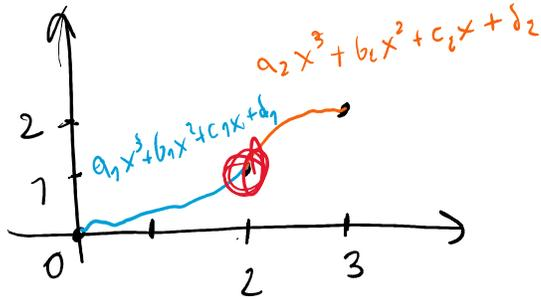
$\Rightarrow f(x) = a_1x^3 + b_1x^2 + c_1x + d_1$ ,  $f'(x) = 3a_1x^2 + 2b_1x + c_1$
