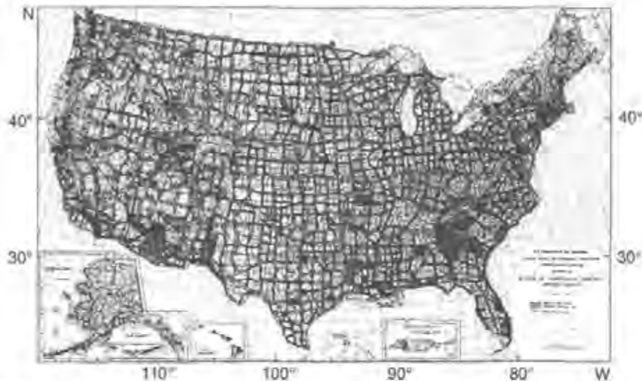
Fig. 7.7. Horizontal control network of the U.S.A. (NAD83), with first and second order triangulation, and traverses, courtesy National Geodetic Survey, National Ocean Service, NOAA
