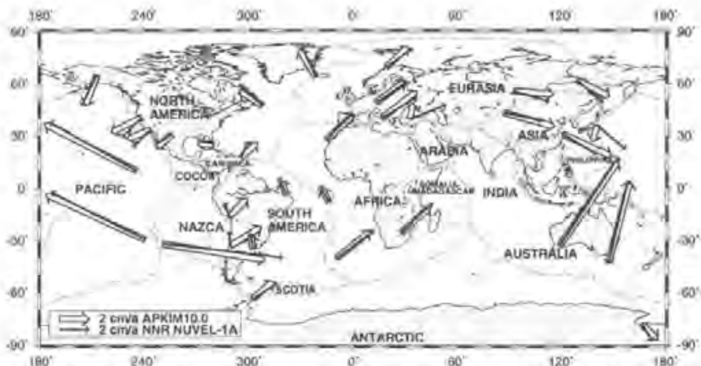
Fig. 8.17. Recent plate motions as determined from geodetic observations (APKIM 10.0 model) and the geophysical model NNR NUVEL-1A, courtesy Deutsches Geodätisches Forschungsinstitut (DGFI), München
