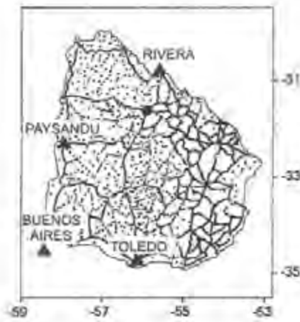
Fig. 7.17. Gravity network of Uruguay, with absolute stations (black triangles), relative stations, and earth tide station (black circle), after SUBIZA et al. (1998)
