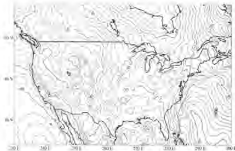
Fig. 6.33. Gravimetric Geoid99 of the U.S.A., contour line interval 2 m (SMITH and ROMAN 2001), courtesy D.A. Smith, National Geodetic Survey/NOAA
