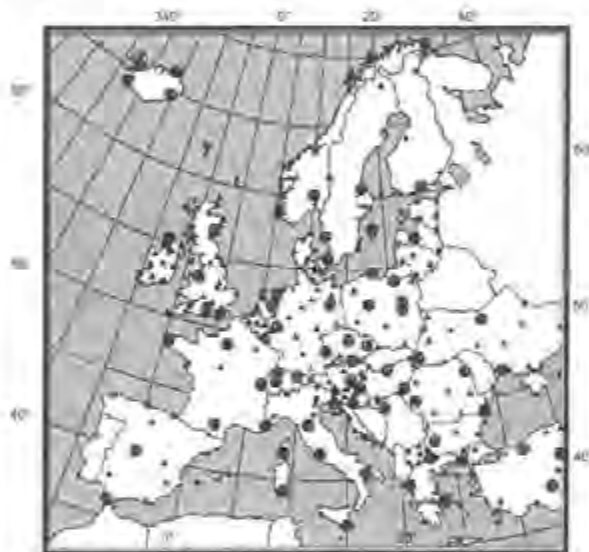
Fig. 7.14. European Reference Frame (EUREF89/97) with permanent GPS stations (status 1999), courtesy BKG, Frankfurt a.M., Germany
