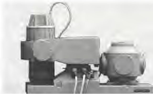
Fig. 5.47. Gravity sensor Gss30 and gyrostabilized platform KT 30, courtesy Bodenseewerk Geosystem, Überlingen, Germany
