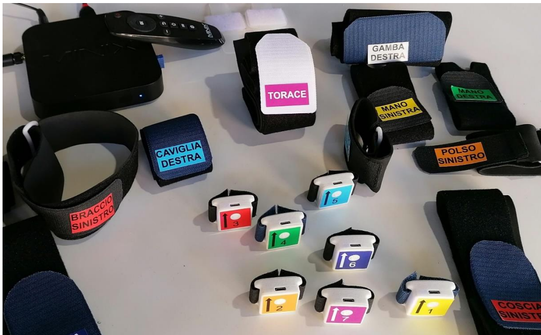
Figure 36: the seven MIMUs and some elastic bands. The thick arrow on the top of each MIMU is useful for the alignment with the longitudinal axis of each body segment.
