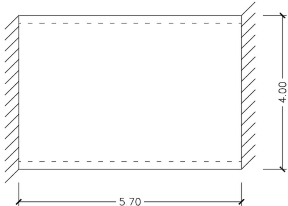
$$\frac{L_{min}}{4} = 1.00 \text{ m} > h = 0.15 \text{ m} \checkmark$$
