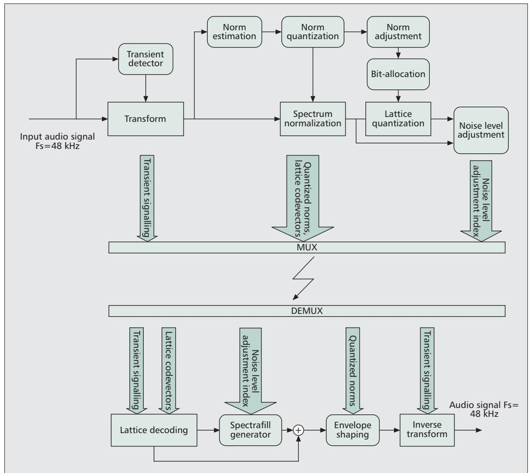
Figure 2. G.719 codec high-level block diagram.
