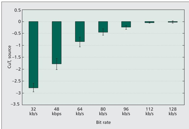
**Figure 4.** Average of difference grades as function of the bit rate (difference between the BS.1116 scores of the source material and the coded material).
