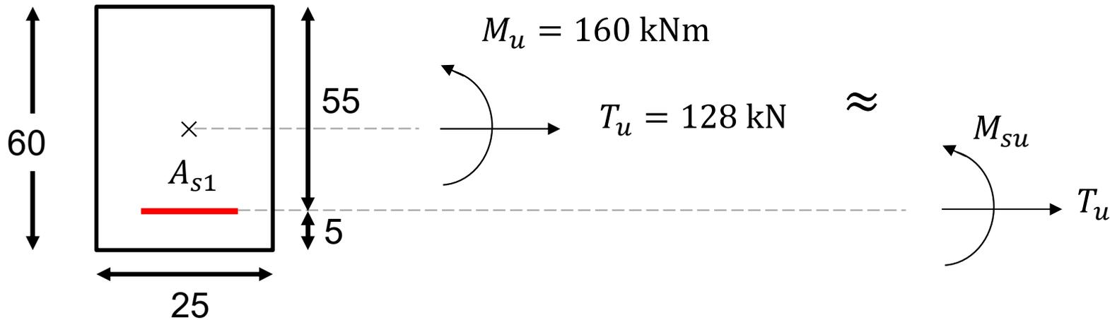
Aplico Ehlers:  $M_{su} = M_u - T_u e_1 = 160 \text{ kNm} - 128 \text{ kNm} \times 0,25 \text{ m} \Rightarrow M_{su} = 128 \text{ kNm}$
