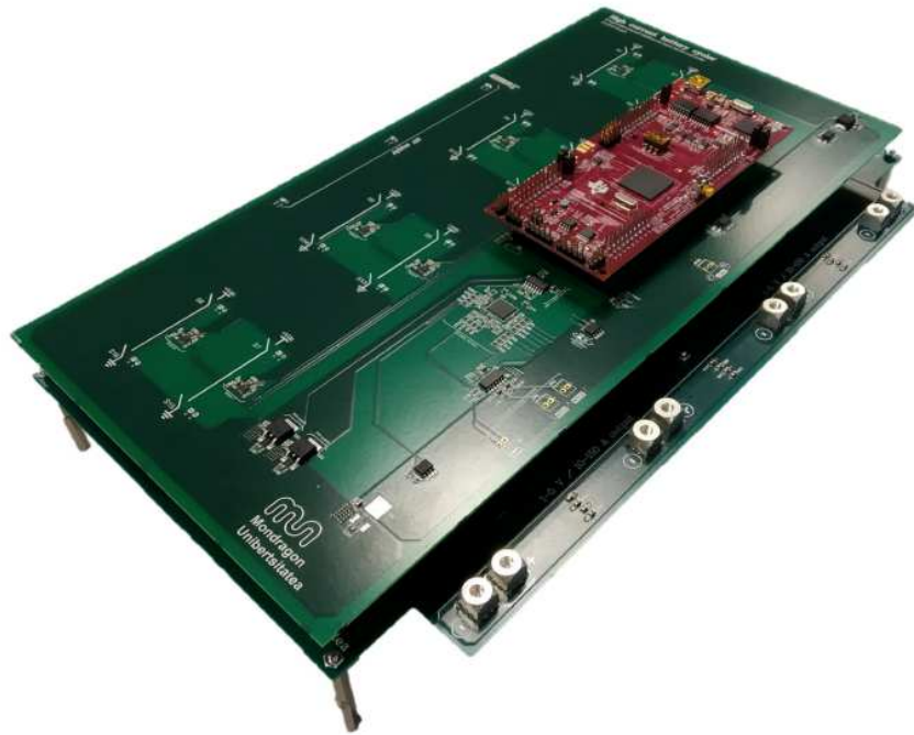
Developed 150A cyclor natural convection
