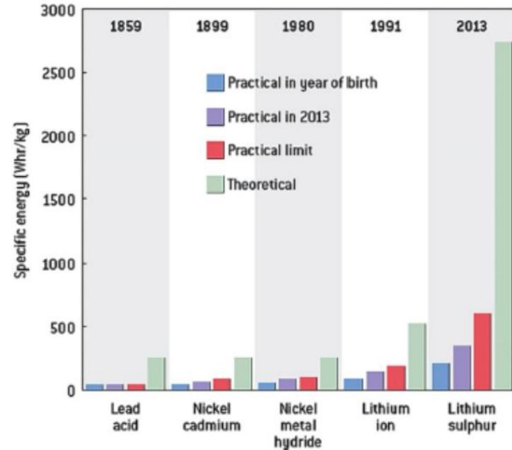
Fig. 11. Specific energy of Li-S battery in comparison with other types [87].
