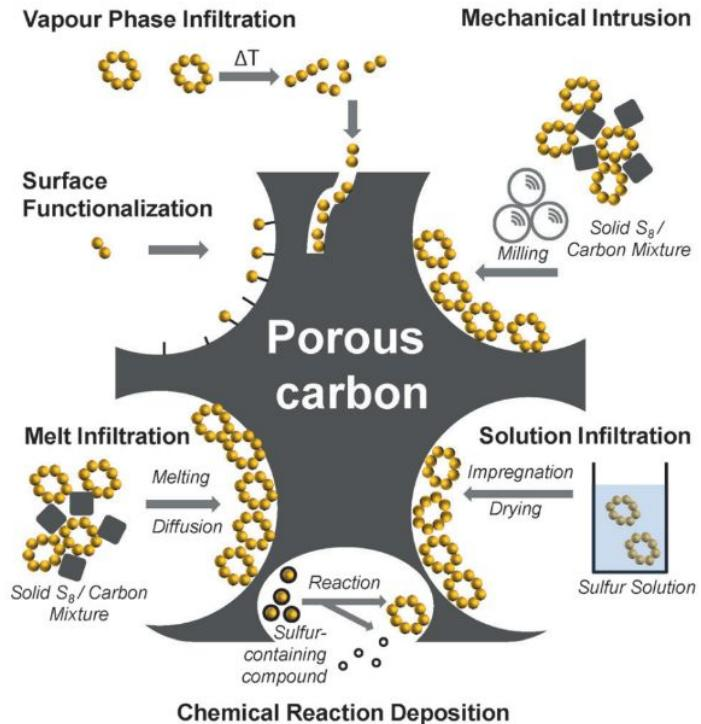
Figure 2. Different approaches for introducing sulfur into carbon.
