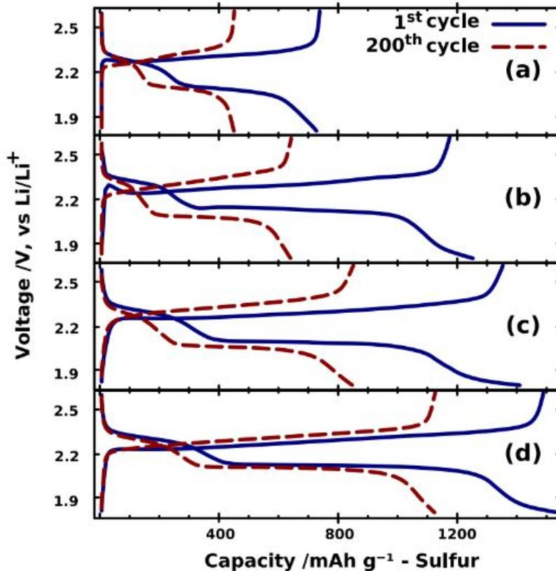
Fig. 3 Charge/Discharge curves of the Li-S cells at 0.2 C of **a** uncoated separator, **b** Sep/C-coated separator, **c** CNF-coated separator, and **d** CNF-coated cathode
