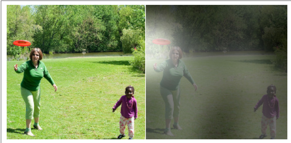
Figure 16-12. Visual attention: an input image (left) and the model's focus before producing the word "frisbee" (right) 39
