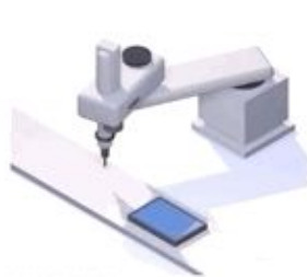
SCARA ROBOT This robot has two parallel rotary joints that allow it to move in a single plane
