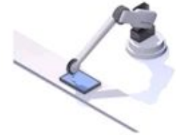
ARTICULATED ROBOT This robot's arm has at least three rotary joints
