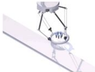
PARALLEL ROBOT The arm of this robot has both a prismatic, or sliding, joint and a rotary joint
