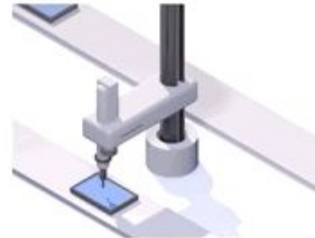
CYLINDRICAL ROBOT The allowable range of motion on this robot is based on a cylindrical coordinate system
