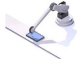
ARTICULATED ROBOT This robot's arm has at least three rotary joints
