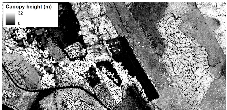
Figure 4.4 A LiDAR based Canopy Height Model showing the canopy height in detail. Lighter colours indicate higher elevations, in this case higher trees. Darker colours indicate lower elevations, and in this case black indicates locations of ground echoes, which can be seen from the road curving on the bottom left or from the rectangular clear-cut areas in the centre of the figure.
