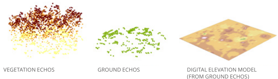
Figure 4.1 Vegetation echoes and ground echoes separated from a 25 meter wide circle, and a digital elevation model interpolated from the ground echoes.
