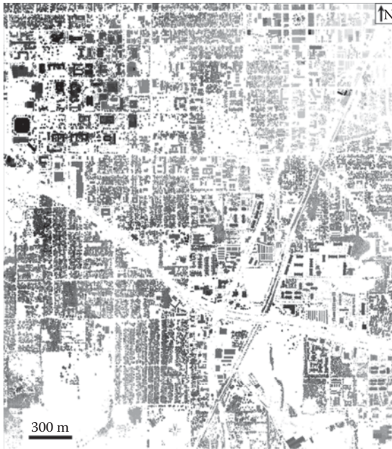
FIGURE 5.3 Non-ground DSM derived from LiDAR data.
