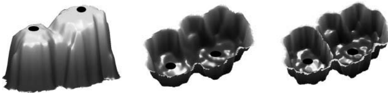
FIGURE 4.15 Marker-controlled watershed segmentation. (Left) CHM, (middle) inverted CHM, (right) inverted CHM with dam built to separate the watersheds. Dark markers are treetops. (Adapted from Chen, Q. et al., Photogramm. Eng. Remote Sens. , 72, 923–932, 2006.)
