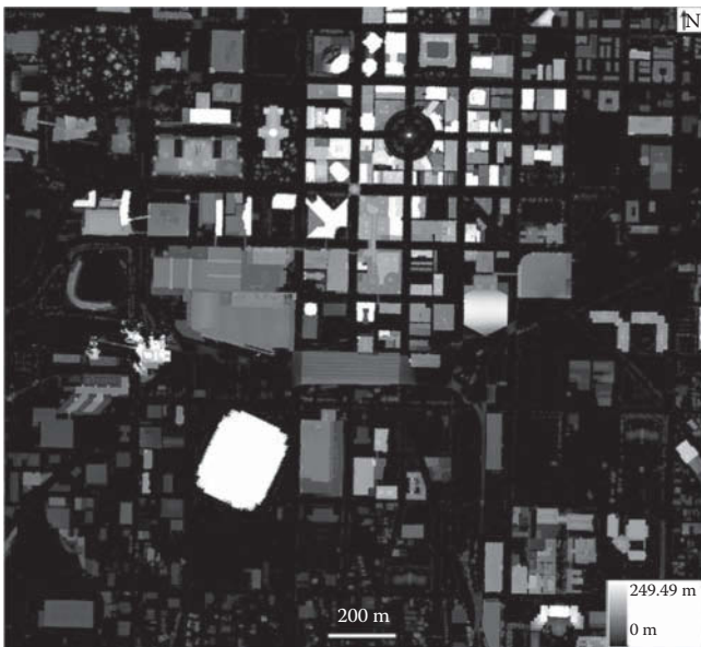
FIGURE 3.12 New DHM obtained from new DSM and DTM.
