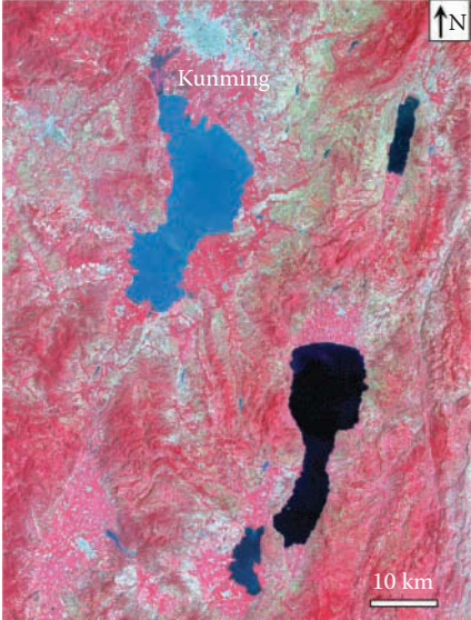
FIGURE 1.3 Color composite of Landsat-5 TM bands 4 (red), 3 (green), and 2 (blue) acquired on August 16, 1992, near Kunming, Yunnan, China.
