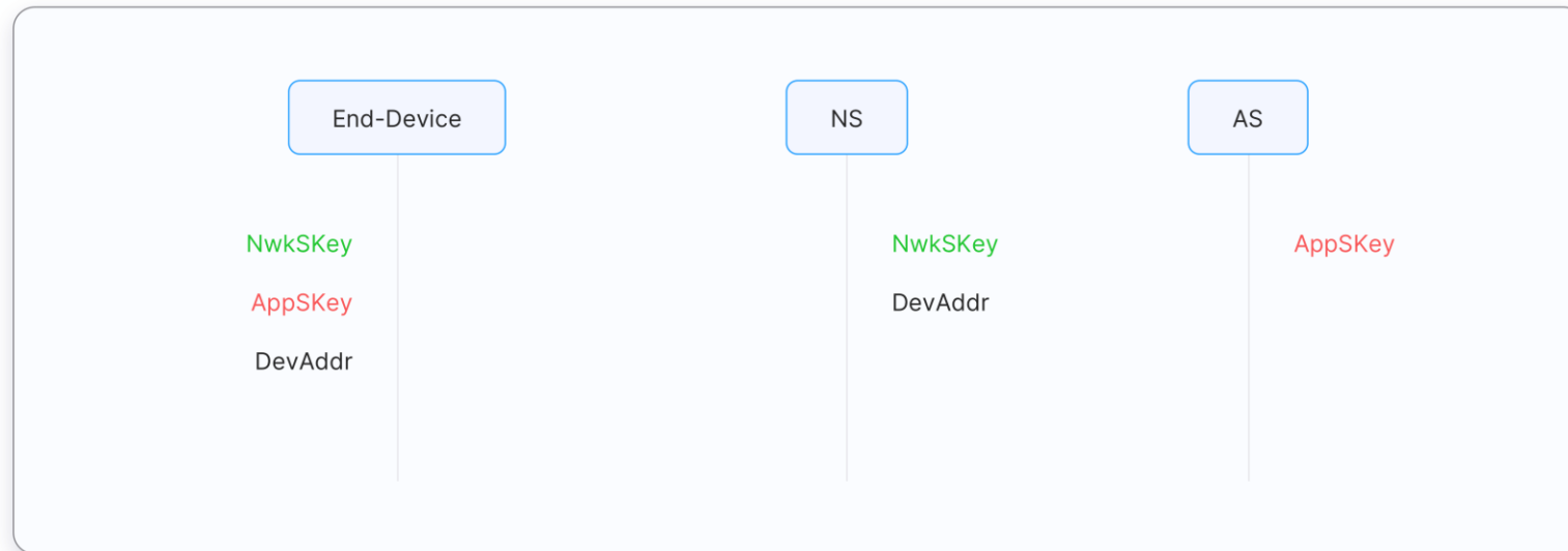
Fig. Activation By Personalisation in LoRaWAN 1.0.x ( https://www.thethingsnetwork.org/docs/lorawan/end-device-activation/ )
