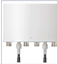
HBXX-6516DS-VTM | HBXX-6516DS-A2M 4-port sector antenna, 4x 1710–2180 MHz, 65° HPBW, RET compatible
