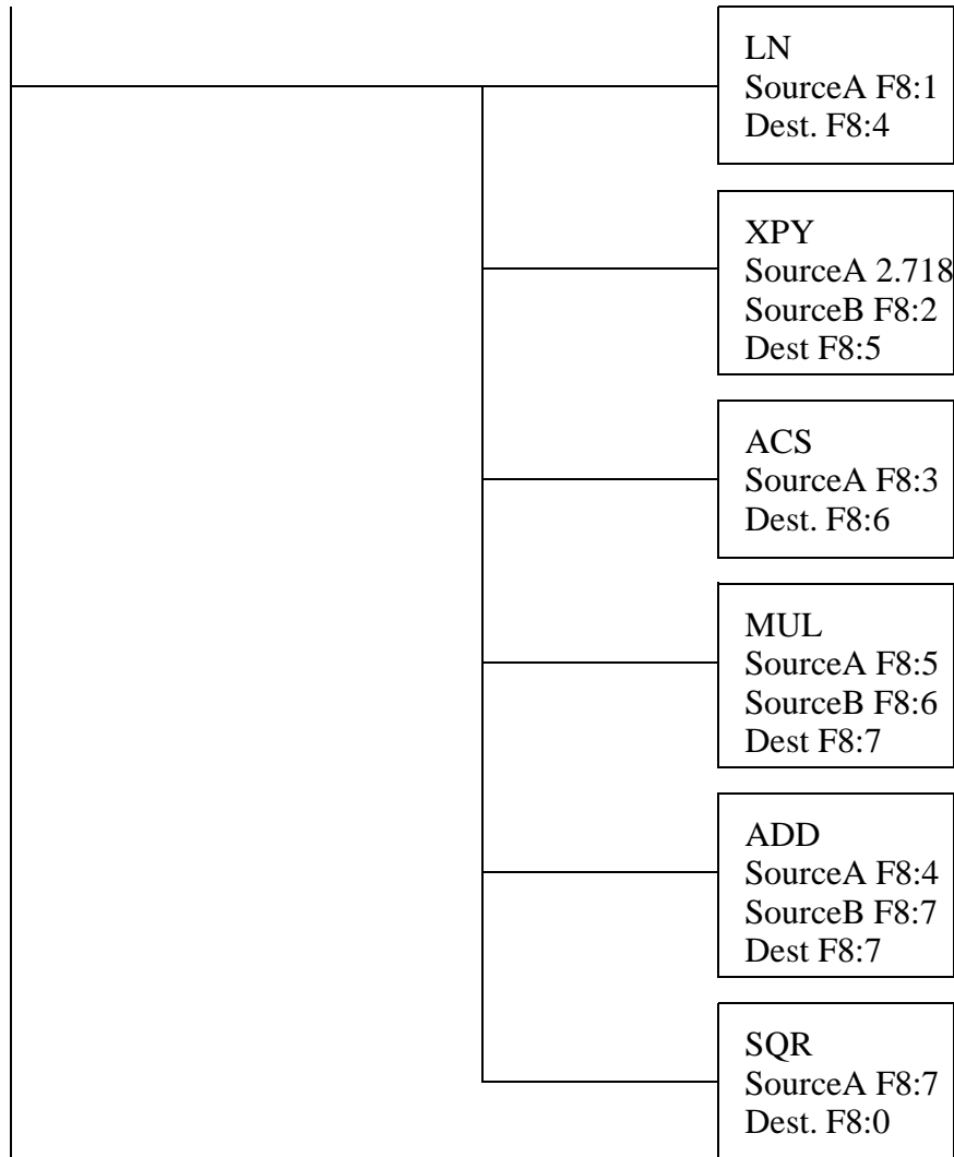
Figure 15.7 An Equation in Ladder Logic
