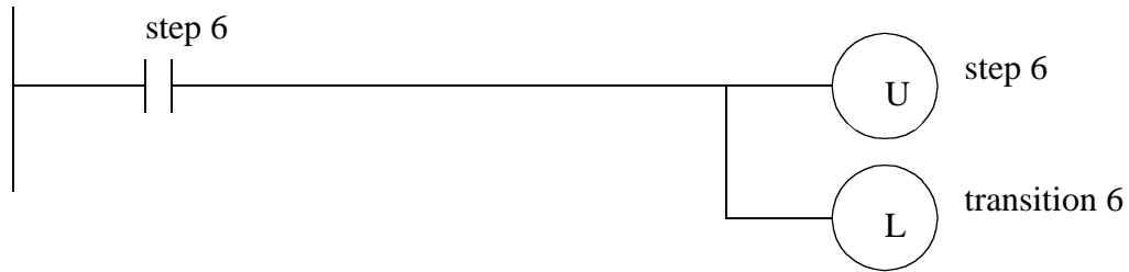
Figure 20.9 SFC Implemented in Ladder Logic
